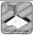
Step 4: Using a 3/16" drill bit, drill pilot hole along the rafter center
