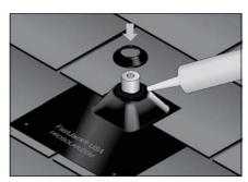
Step 7: Apply 1/4" bead of sealant (Geocel 4500) and compress with aluminum collar
