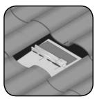
Step 8: After bolting the base to the roof, slide the upper carriage under any portion of the crown (high point) of the tile."
