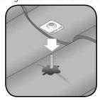
Step 12: Unbind nuts and remove from stud. Apply sealant around stud at tile opening and compress with Stainless Steel flashing (included) until seated.
